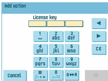
2. Use the keypad to enter the license key code that you received from the supplier to activate the relevant option on this machine.
