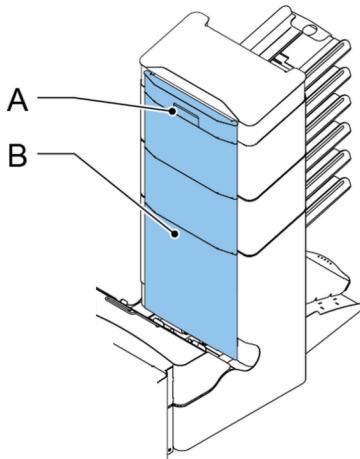
1. Pull the vertical transport hand grip **A** upward to open the vertical transport cover **B**.
