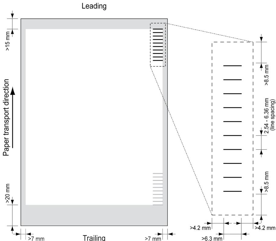
Minimum line thickness of a mark: 0.2 mm (0.008 inch)
