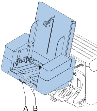
The High Capacity Vertical Stacker can be used to stack filled envelopes. The vertical stacker can store up to 325 filled envelopes. In case you have a High Capacity Vertical Stacker, install it as follows on your system:
