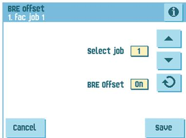
2. Use the
