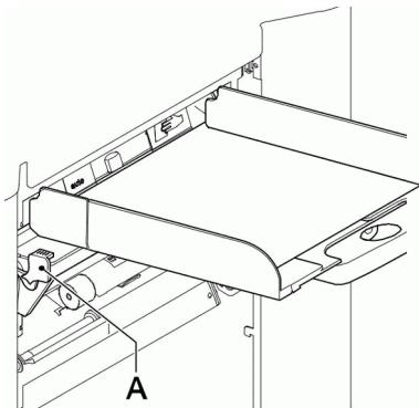
2. Lift the document feed tray upwards to unhook it and then pull it out from the feeder.
