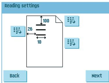
In this menu you can define the location and the width of the OMR code. The position from top should be between 15 mm (0.6 inch) and the document length minus 20 mm (0.8 inch). If you press **[Next]**, you can load an OMR sheet to verify the OMR settings. The system processes the OMR sheet and shows the read marks. The information button shows the interpretation of the marks.
