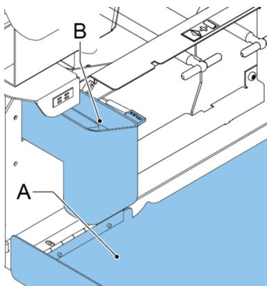
2. Fill the reservoir **B** to the "Max" lip with sealing liquid.
