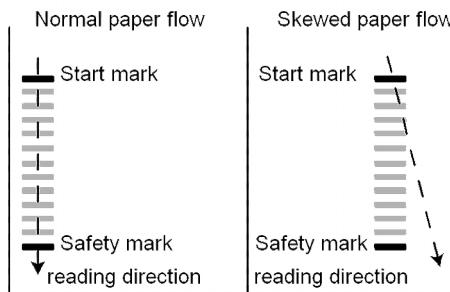
The minimum code is one mark in one line (insert). However for reliability it is advised to use at least 2 marks. The first line is the start mark. A mark printed on the second line means insert. No mark on the second line means accumulate.
