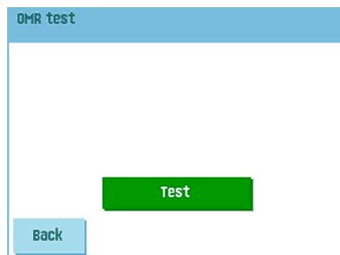
2. Press the [Test] button to start the OMR test. After the test is finished, the Result screen appears.
