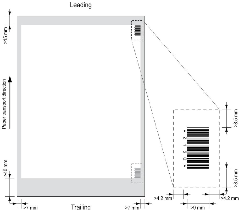
Minimum line thickness of a bar: 0.25 mm (0.01 inch)
