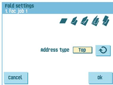
Select the Address type. In case the system is equipped with the optional bottom address application you can switch between Top and Bottom address position.
