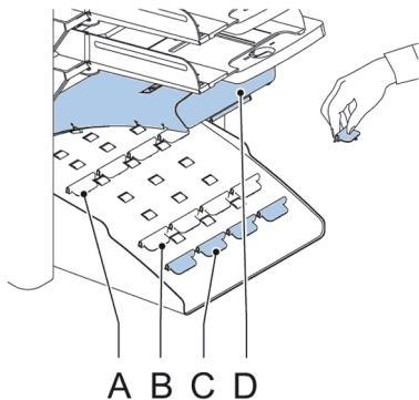
When a job is selected in which a different stopper position has been programmed, the operator has to put the document stoppers in the correct position as indicated by the display.
