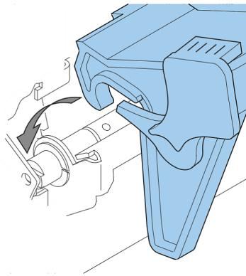
4. Move the document feed tray towards the machine and move the hooks over the mounting points (on both sides).
