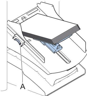
2. Adjust the side guides by turning the thumb wheel **A** so the documents/BREs just fit and can move without resistance.
