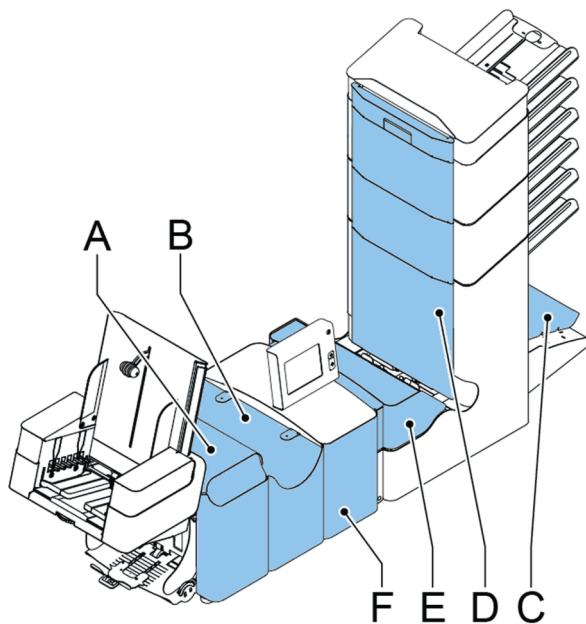
**A** - loc cover, to reach the sealing and exit area
