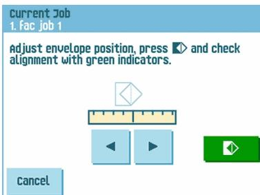
2. Use the arrows beneath the ruler to adjust the envelope position.
