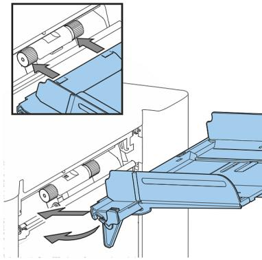
2. Place the front end of the document feed tray underneath the two black rollers.
