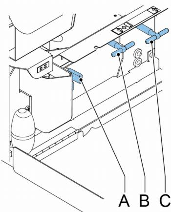
If needed, envelopes can be transported manually to the insert table or lower envelope track by means of handle **C**. To transport a mail set manually, turn handle **B**.
