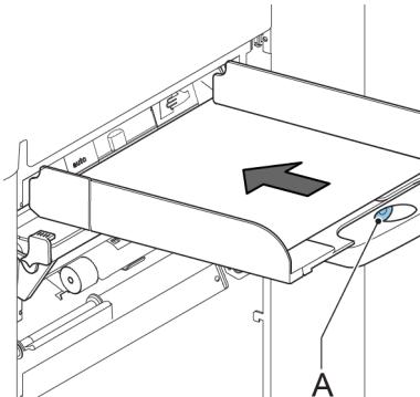
2. Place a document on the feed tray and slide it about 60 mm (2.4 inch) into the system (turn the knob A counter clockwise if the separation is set too narrow).
