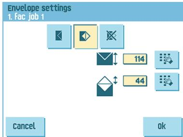
In the top of the screen, three selection buttons are displayed, from which one can be selected. The selected settings button will be highlighted.
