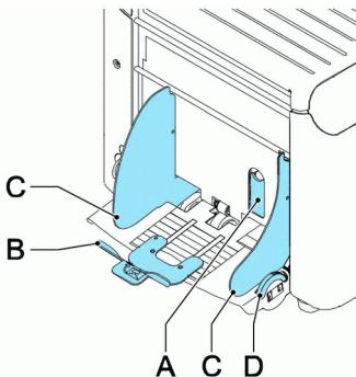
2. Put a small stack of envelopes between the side guides.
