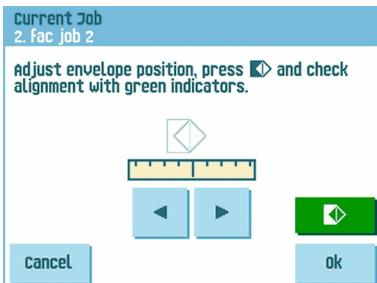
4. Press the **[OK]** button to accept the new alignment.
