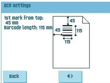
4. In the BCR settings screen, confirm that all settings are read correctly. Note that this screen consists of two parts. Use the arrows at the bottom of the screen to navigate between the two parts of this screen.
