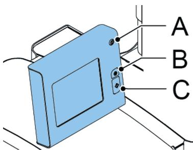
The control panel consists of the touch screen and the following buttons:
