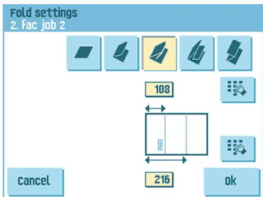
To change the fold positions press the button next to a fold. Enter the required position of the relevant fold.
