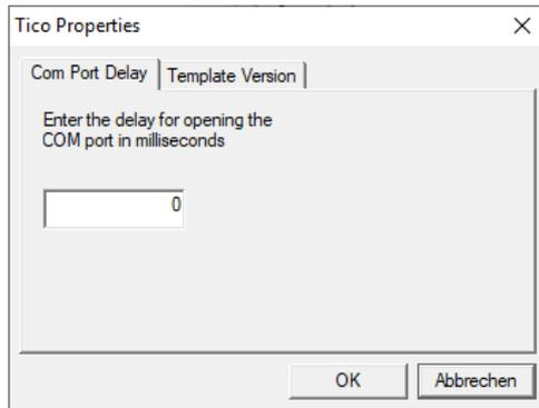
The Template Version specifies the project structure in the FP Gateway. FP InovoLabs periodically releases new Firmware versions with new functions which may require new commands and registers to be merged or added. To prevent compatibility issues the chosen template version has to match the firmware version of the device.
