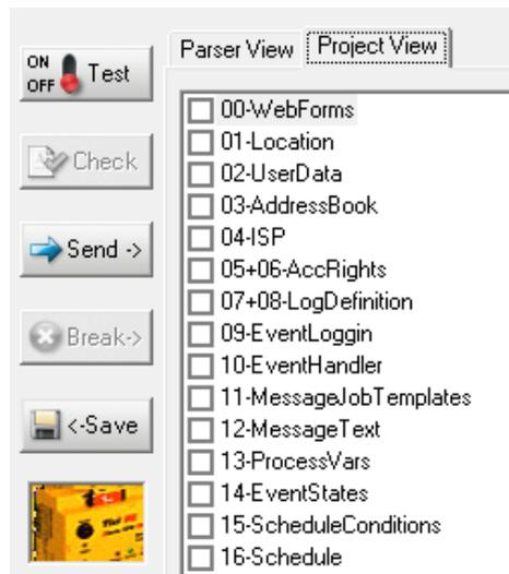
Right click on an entry in the Project View opens a context menu to remove the marked database from the project. The database will be hidden and may later be added back to the project with its old content.
