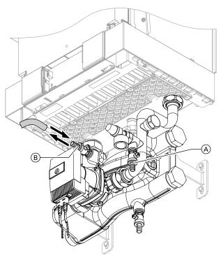
Fig. 19 Connection set with integral low loss header
