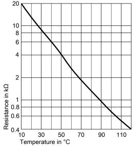
Fig. 46 Sensor type: NTC 10 kΩ
