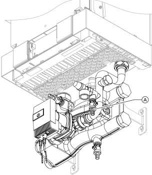
Fig. 18 Connection set with integral low loss header
