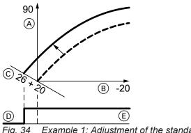
Fig. 34 Example 1: Adjustment of the standard set room temperature from 20 to 26 °C
