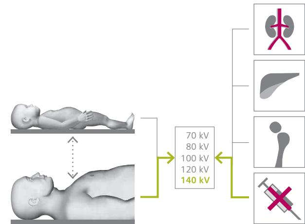
**Example 2:** For a non-contrast examination of a large patient, CARE KV suggests a scan with 140 kV and sets the other values accordingly.
