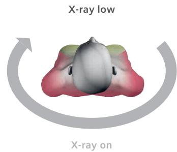
X-CARE reduces the tube current close to zero within a certain range of projections, minimizing direct exposure for highly dose sensitive body regions.
