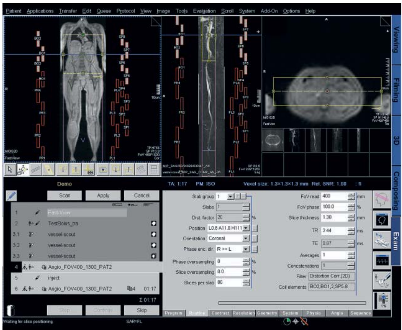
[ Figure 5 ] VesselScout and planning of the syngo TimCT 3D FLASH MRA sequence. The coronal view of the FastView localizer and the sagittal view of the Vessel Scout together serve as reference for planning of the coronal slab of the 3D FLASH MRA sequence. Since this is a continuously moving table protocol, the user only has to assure that the MRA volume covers the vessels of interest over the full lengths of the VesselScout. No further planning steps are required.
