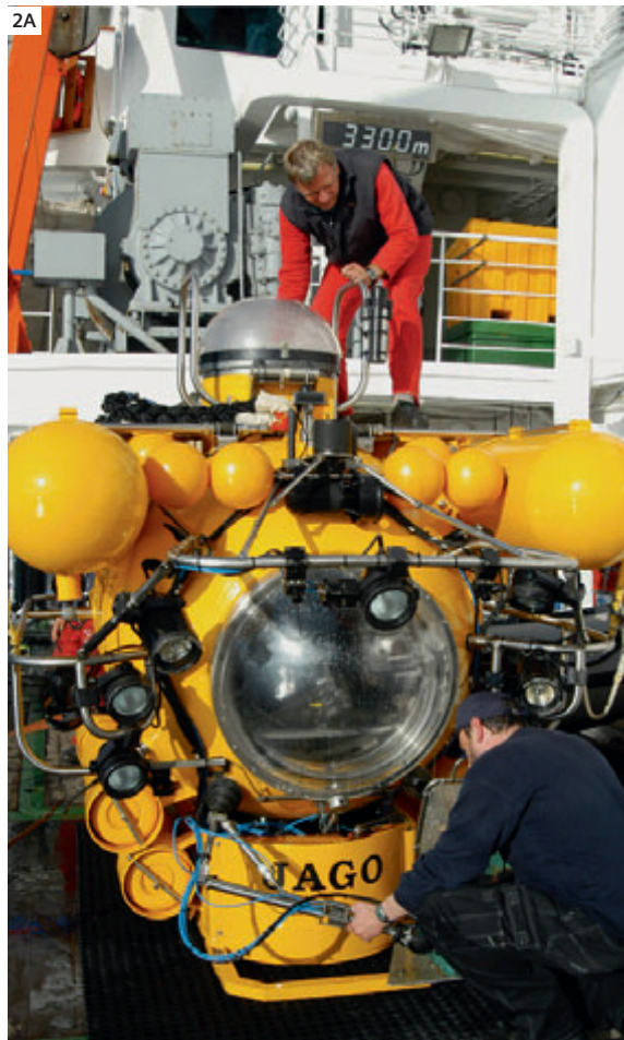
2 Oceanographic research vessel R/V Poseidon cruising the north-Norwegian Stjernesund Fjord, home to the world's most northern corals (Fig 2B). Manned submersible JAGO aboard the vessel, being prepared for a dive in the 400 m deep fjord (Fig. 2A).
