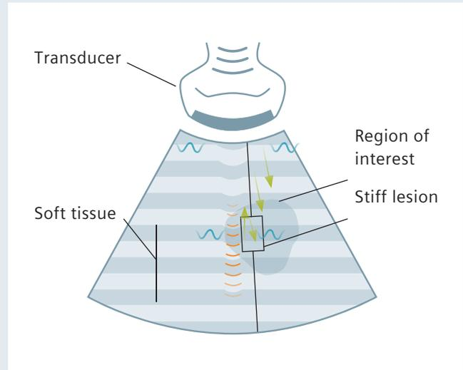
**Figure 9:** Virtual Touch quantification utilizes an acoustic push pulse (orange) to generate shear waves (blue) through a user-defined region of interest. Detection pulses are applied in multiple locations and reveal arrival time, allowing calculation of the shear wave propagation speed.
