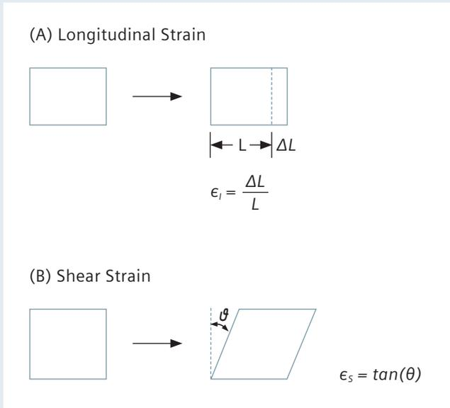
Figure 3: (A) Longitudinal and (B) Shear Strain.
