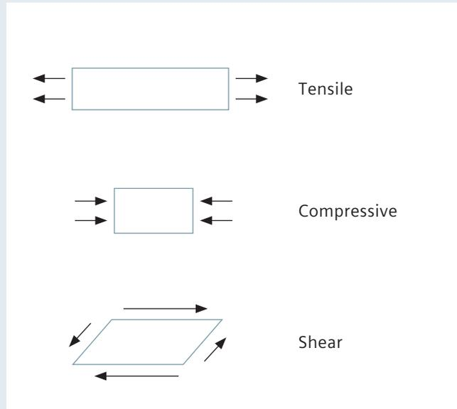
Figure 4: Stress and Strain.
