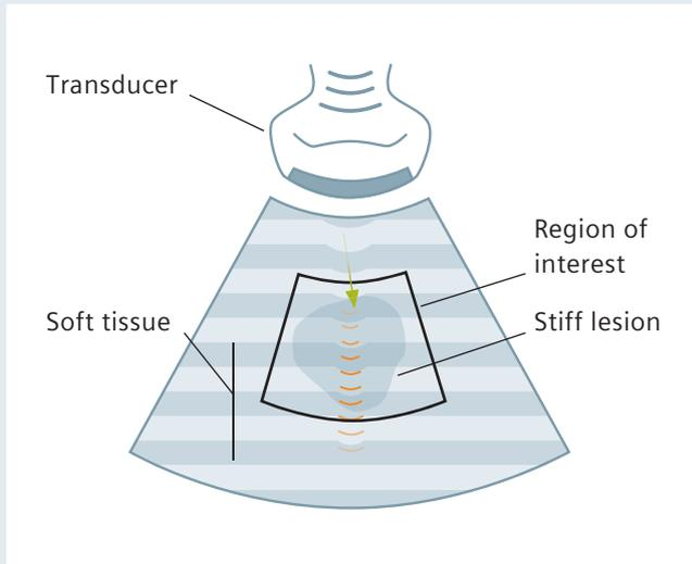
**Figure 8:** Virtual Touch imaging utilizes acoustic push pulses (orange) and detection echo (green arrow), sequenced across a user-defined region of interest, to generate a displacement map depicting the relative stiffness of tissue.
