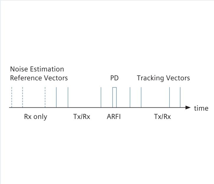
**Figure 12:** Data acquisition sequencing for a pair of ARFI excitation and detection locations. In the noise estimation segment there is no transmit (Tx), and the received echo signal (Rx) is used to estimate the noise level. In both reference vectors and tracking vectors, wide band transmit and receive is used to obtain the echo signals, and these signals are used to estimate the tissue displacement.
