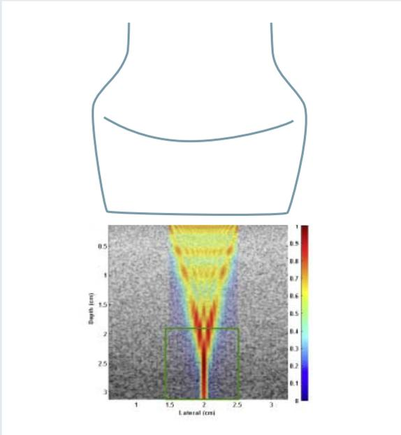
**Figure 10:** Illustration of focused ultrasound beam (color overlay in the echo image), region of interest (green rectangle box), and ultrasound transducer, which generates the focused beam and receives echo signal. The colors represent the relative acoustic intensity levels in the demonstrated beam, with the solid dark red color indicating the highest intensity level, while the light and transparent purple color represents lower intensity levels.
