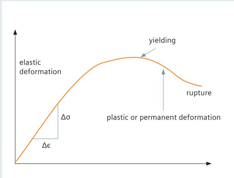
Figure 5: Relationship between Stress and Strain in Material.
