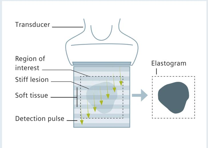
**Figure 7:** Tissue strain is induced by minimal **mechanical compression** with the transducer or cardiac pulsations and respiration. Detection pulses track displacement, which are used to derive a strain image in gray scale or color-coded display.
