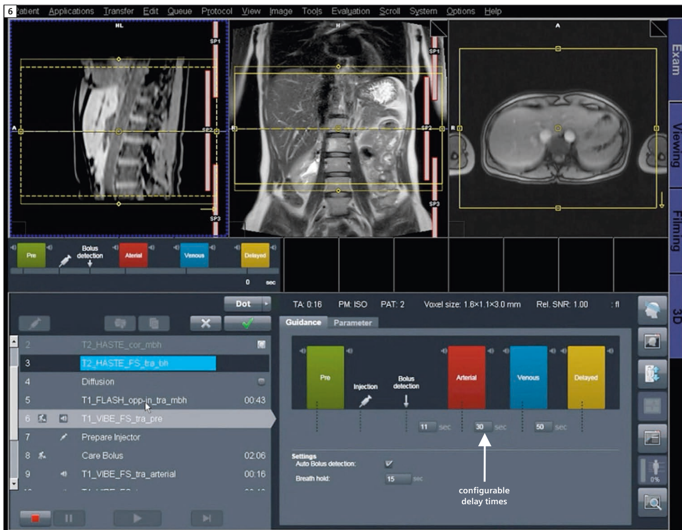
6 Example of the Abdomen Dot Engine user interface showing the guidance view that allows global planning of delay times within a dynamic contrast enhanced liver MRI protocol.
