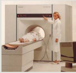
First actively shielded 1T system
