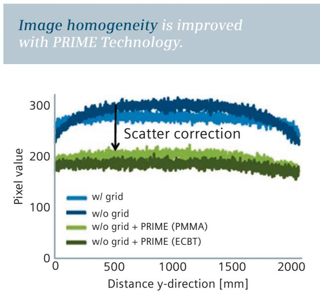
Figure 8: Improved image homogeneity with PRIME Technology has the potential to overcome cupping artefacts, i.e. intensity bias (phantom study) [20]. The Y-direction is parallel to the chest wall.
