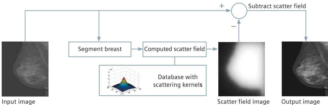
**Figure 4:** Simplified illustration of the PRIME algorithm for scatter correction [13]. PRIME Technology estimates and subtracts the low-frequency component of the scattered radiation in a process of convolution, using a database with 2D scatter kernels. Effects of the high-frequency component of the scattered radiation are reduced indirectly through a larger amount of primary radiation reaching the detector with gridless image acquisition.
