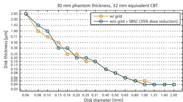
Figure 6: Pair of contrast-detail curves (log-log plots) illustrating similar image quality for grid-based acquisition and dose-reduced gridless acquisition plus PRIME Technology (phantom study) [13].
