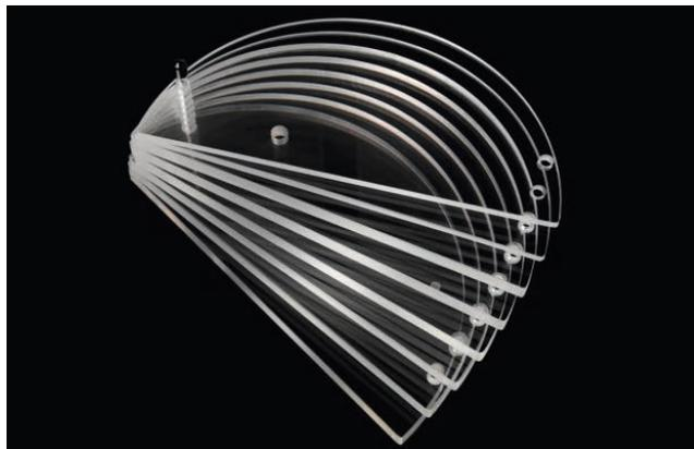
Figure 3: Example of a PMMA phantom.
