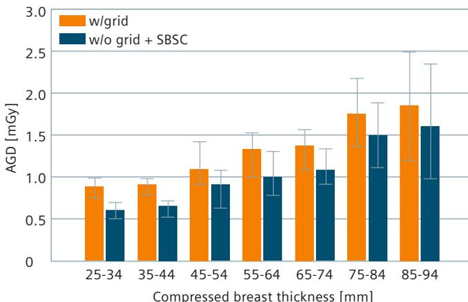
**Figure 7:** The absolute AGD reduction with gridless acquisition plus PRIME Technology was 0.26 ± 0.06 mGy (mean ± SD) and similar across CBT ranges (clinical study) [13].
