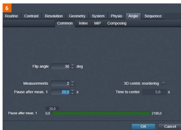
Figure 6: Two measurements are configured with a 20-second break after the first scan.
