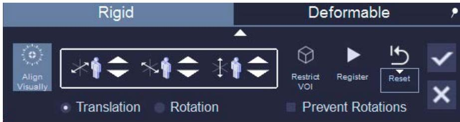
Figure 1: Control panel offers options for translational and rotational shifts of the data set in addition to visual alignment and restriction of the registration to a Volume-of-Interest (VOI).a
