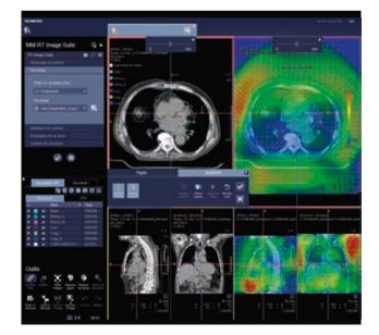
Figure 5: Example of deformable registration results visualized with vector map and deformation magnitude color map
