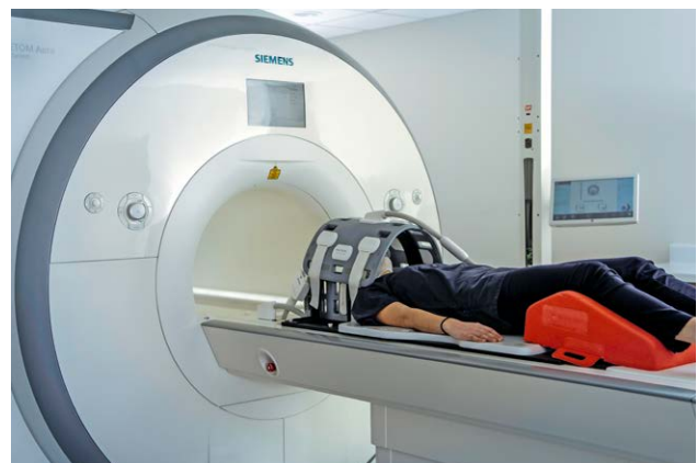
1 Example of patient positioning for MR Brain acquisition for radiation therapy planning on 1.5T MAGNETOM Aera.
