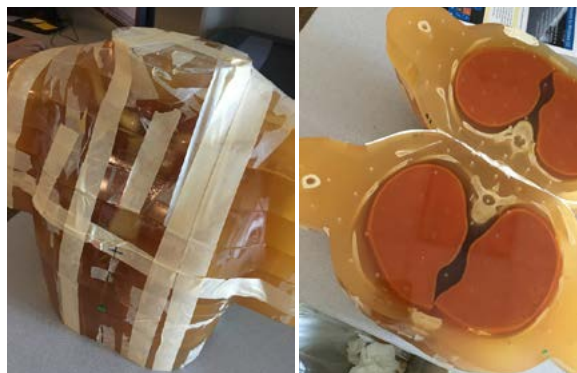
Figure 11 Alderson RANDO phantom used to verify DD-based dose calculations in Raystation
