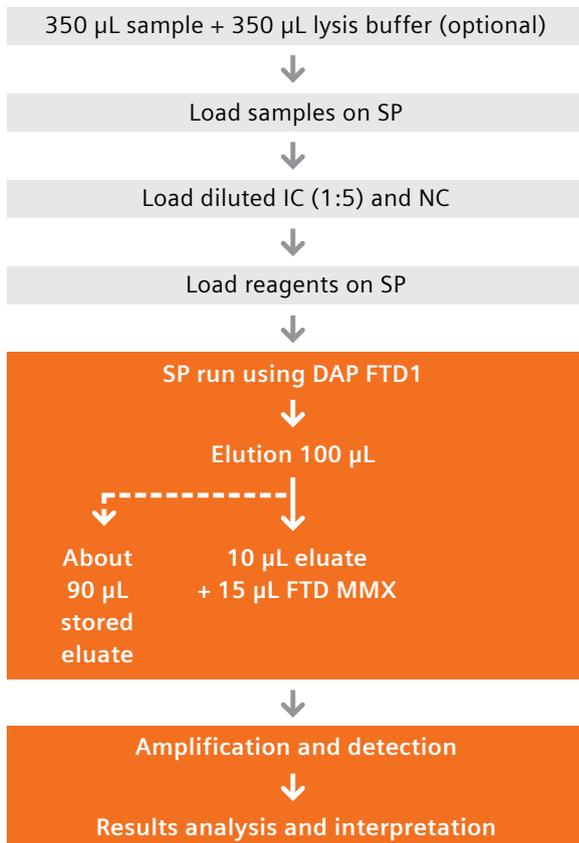
**Figure 3.** Schematic protocol and workflow on the VERSANT kPCR Molecular System.
