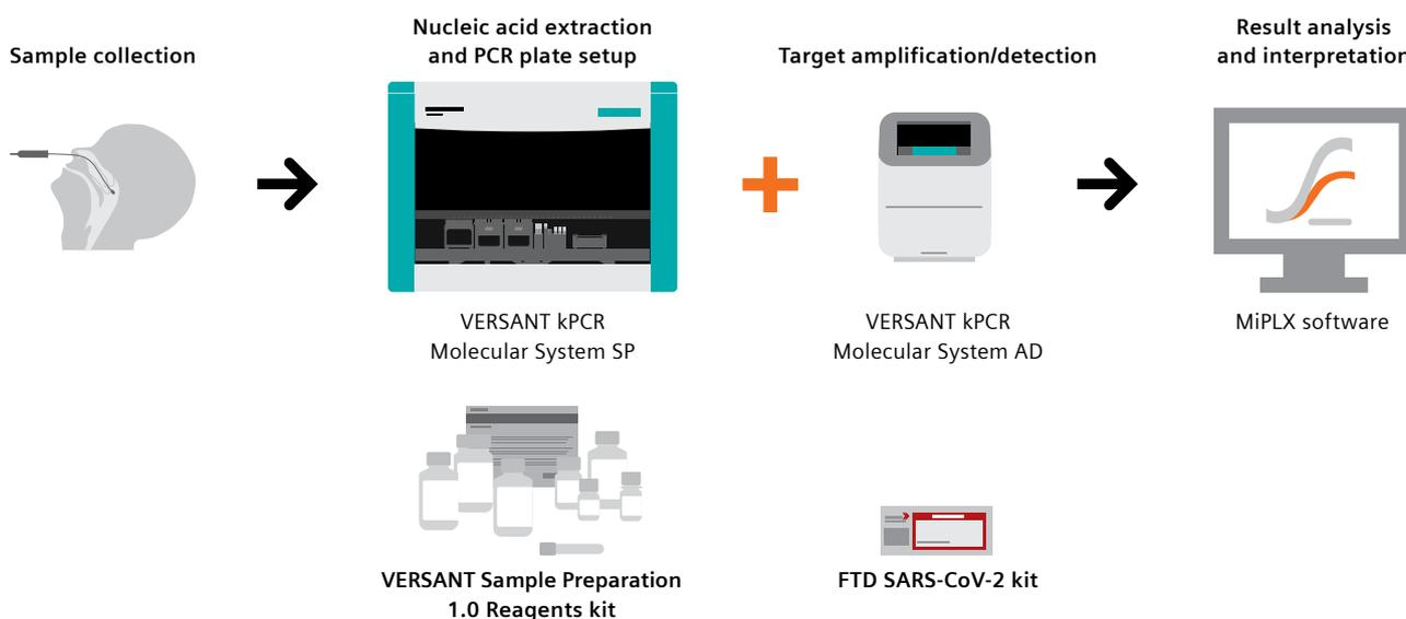
**Figure 2.** VERSANT kPCR Molecular System workflow for the FTD SARS-CoV-2 Assay.
