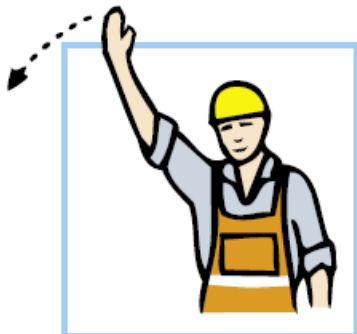
DRIVE OFF initiating or continuing a driving motion according to the previous direction signal
