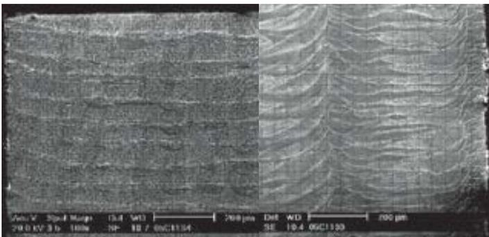
*Left: build with 20  $\mu\text{m}$  layer thickness throughout the entire part.
