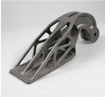
*Lightweight turbine cover door hinge for Airbus A380
