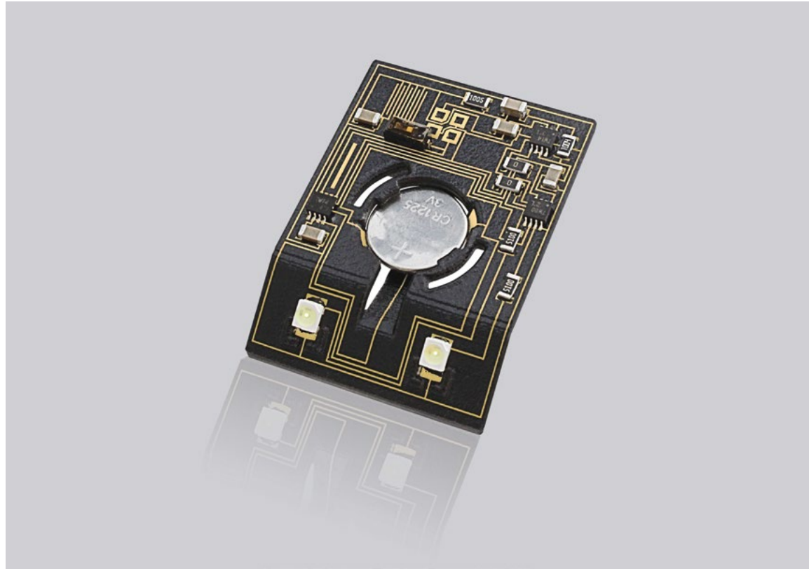
Highly functional, fitted circuit carriers made of PA 3200 GF by using additive manufacturing technology. (source: Beta LAYOUT)
