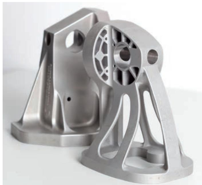
*Further example of improved part design: prototype of a topology optimised Airbus A380 bracket made of stainless steel powder produced via DMLS with conventional bracket behind (Source: EADS).*
