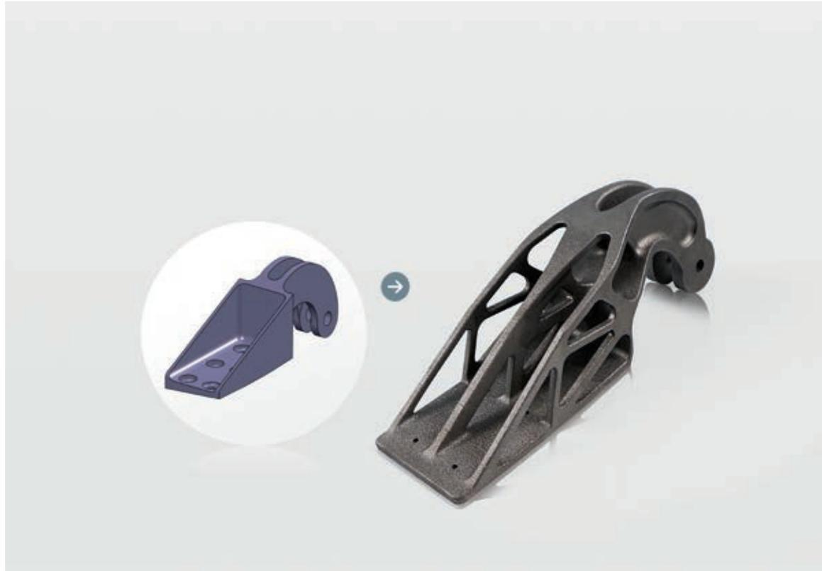
*Graphic of the conventional design of the assessed steel cast bracket (left) and titanium bracket with optimised topology made by using DMLS technology (Source: EADS)*
