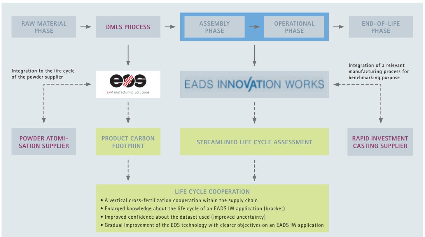
Figure 17: A life cycle cooperation approach by EADS IW and EOS on an aeronautic application
