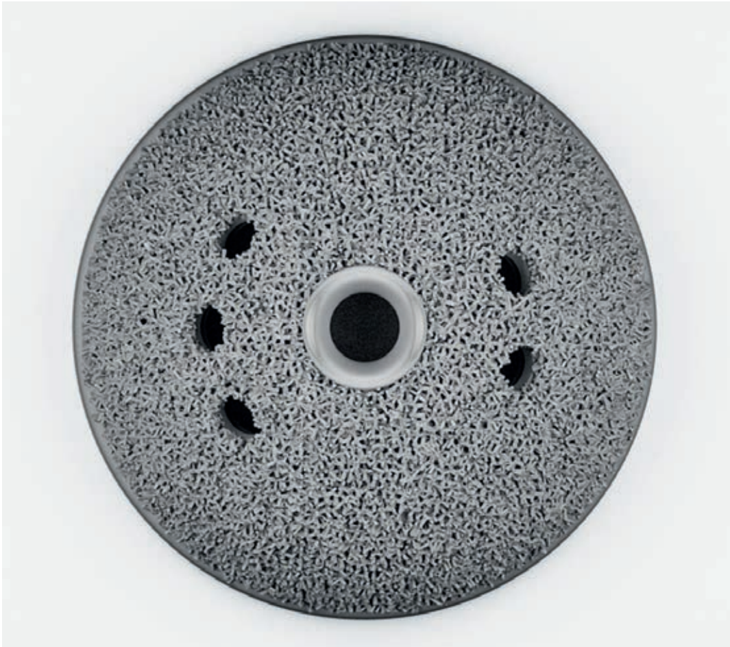
Fig. 5: Hip implant with lattice structures for improved osseointegration. Additive Manufacturing in a single step using EOSINT M 280
