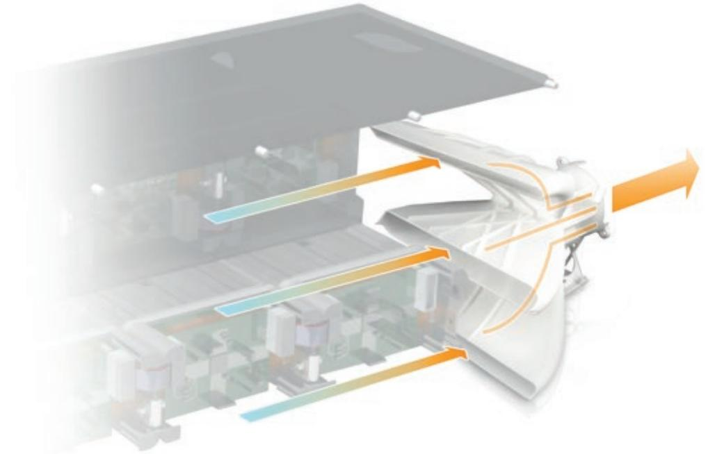
*The complex and lightweight component for dissipating heat reduced the top temperature within the container from 80 °C to just 50 °C. This translated to an increase in cooling performance of over 100% (courtesy of DHBW Engineering Stuttgart).*
