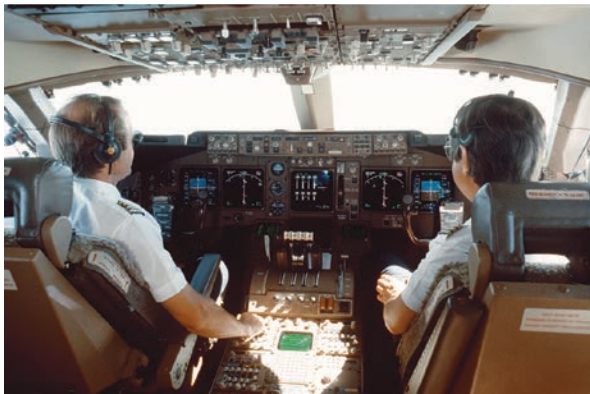
The 747-400 flight deck is much roomier and simpler, with many of the previous generation of instruments now integrated into a few monitor screens. The number of instruments has been reduced to less than 400.
