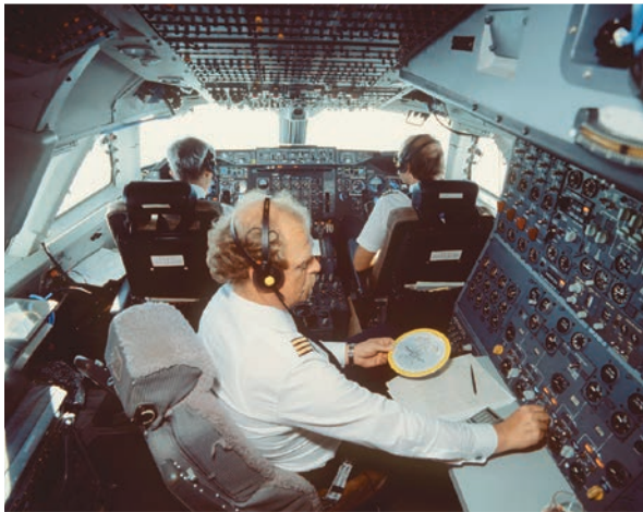
Two cockpits – and two epochs in aircraft technology. Above, the flight deck in the Boeing 747-200 with the third seat for the flight engineer, and more than 1,000 instruments, dials and switches.
