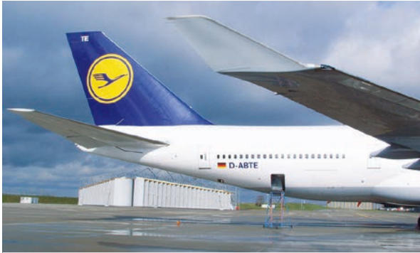
Winglets on the wing tips reduce drag and save fuel (here on a Boeing 747-400).
