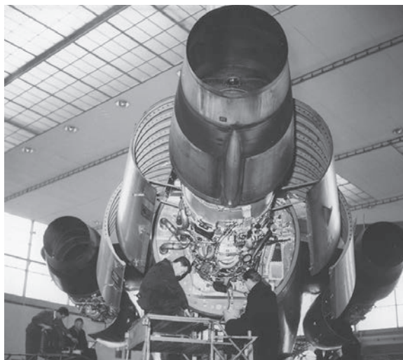
The centerline engine in the Boeing 727 rear fuselage under maintenance.
