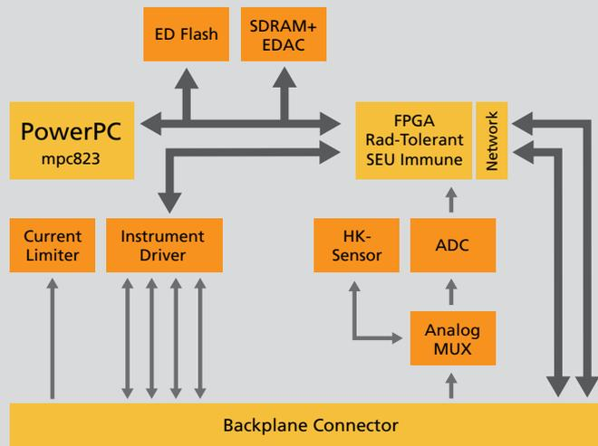
FOKUS is employing an FPGA because it is freely programmable and can thus be adapted to the various interfaces. The FPGA in turn is built with a triple redundancy (TMR-Triple Module Redundancy).
