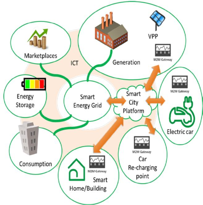
Figure 3. System model of the electricity grid using the Smart City platform to accommodate new services like searching for the nearest free electric car re-charge point
