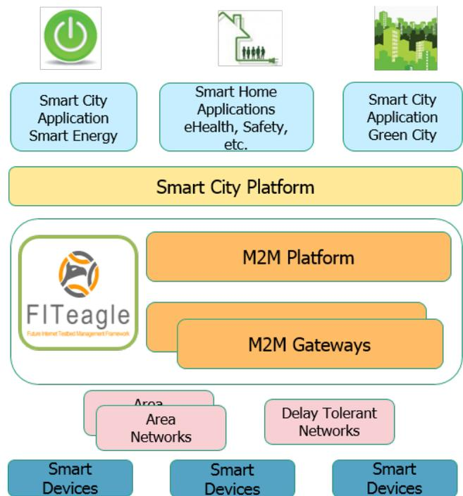
Figure 1. Smart City Reference Architecture.
